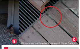
A Embers that pass through deck board gaps will land on the ground, or on combustible materials stored under the deck, as shown during this IBHS test.
